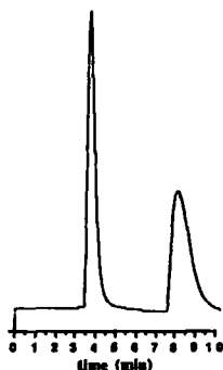
Figure 2: Actual chromatogram showing the separation of underivatized naproxen enantiomers using CSP 2. k'_{(R)} = 1.71 ; k'_{(S)} = 5.01 ; \alpha = 2.93 . Conditions: Flow rate = 2.0 ml/min, mobile phase = 20% 2-propanol in hexane containing 1 g/l ammonium acetate, UV detection at 254 nm, ambient temperature.
